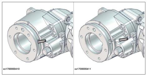
When calibrating axis 6, push in the calibration tool into the turning disc until the snap ring engages, no further.
