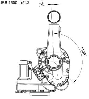
2.4.3 Installation of additional mechanical stop on axis 2 *Continued*
