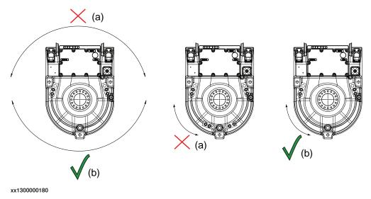
(a) The additional stop pin does not manage the extra gravity force in this restricted working area (for tilted or wall mounted robots).
