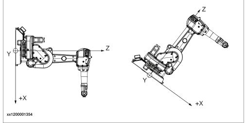
Negative directions in axis 1 have extra gravity force (tilted or wall mounted robots)
