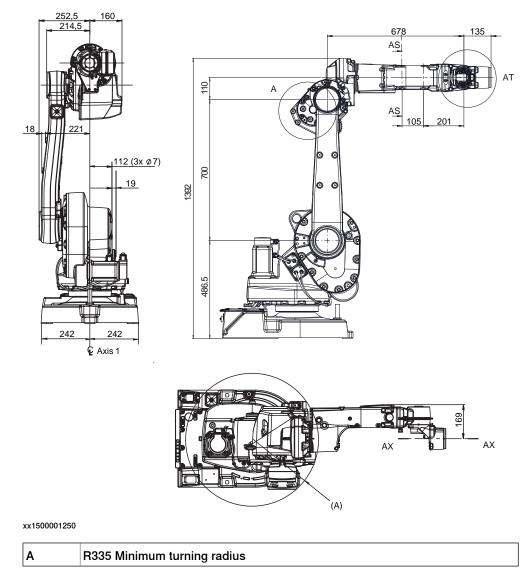
2.3.7 Fitting equipment on the robot (robot dimensions) *Continued*
